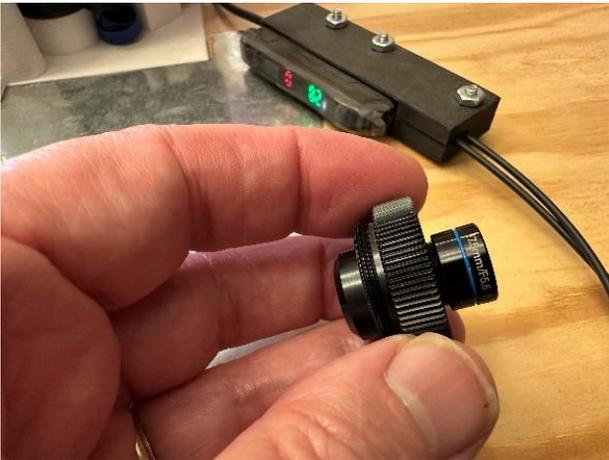
If you are scanning a 16mm Film, start with a 5mm Extension. If you are doing 8mm, try two of them. 35mm might not need any extensions. Use the magnets to hold the Glissade to the metal plate and to hold the camera in place at the bottom.
