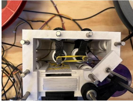
There is no official way to set up the turntables to move the film. A small hole can be drilled near the center shaft and a pin can be inserted. This will work for the reel risers as well as the base. You can also wrap wire through the holes and the reel to secure it.
