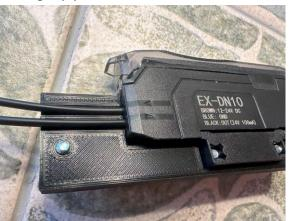
Hot glue the light pipes to one side of the housing and put the other side of the housing on while the glue is still soft and screw the two sides together with a #6 nut (you can also just use tape to keep the two sides together). Set the SEL/M switch to the "M" Position. The sensor is complete.
